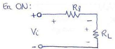
$$i = \frac{V_m \sin \omega t}{R_f + R_L} \rightarrow i R_f = V_D$$
