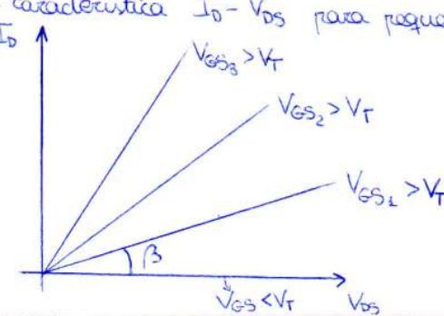
$$I_D = g_{d0} \cdot \frac{V_{DS}}{r_d}$$
