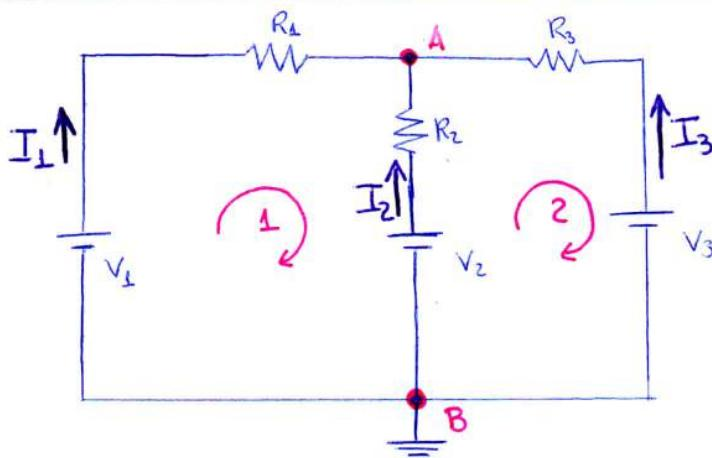
$$\begin{aligned}V_1 &= 12 \text{ V} \\V_2 &= 2 \text{ V} \\V_3 &= 20 \text{ V} \\R_1 &= 2 \text{ k}\Omega \\R_2 &= 1 \text{ k}\Omega \\R_3 &= 3 \text{ k}\Omega\end{aligned}$$
