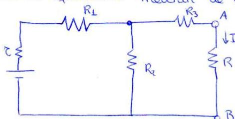
$$\begin{aligned} r &= 1 \Omega \\ R_L &= 9 \Omega \\ R_2 &= 20 \Omega \\ R_3 &= 40 \Omega \\ \text{fém} &= 0,5 \text{V} \end{aligned}$$
