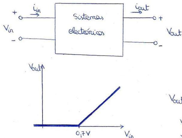
$$V_{out} = f(V_{in})$$
