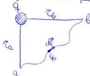
$$W_{a \rightarrow b} = U_b - U_a = \int_a^b -\vec{F} d\vec{\ell} = - \int q_0 \vec{E} d\vec{\ell} = k q_0 q \left( \frac{1}{r_b} - \frac{1}{r_a} \right)$$
