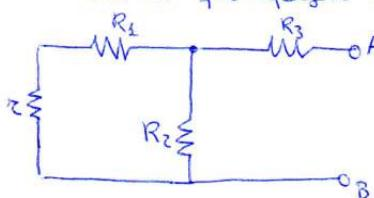
$$\begin{aligned} R_{th} &= (R_2 \parallel (R_1 + z)) + R_3 = \\ &= \left( \frac{1}{R_2} + \frac{1}{R_1 + z} \right)^{-1} + R_3 = \\ &= \left( \frac{1}{20} + \frac{1}{10} \right)^{-1} + 40 = 46,67 \Omega \end{aligned}$$
