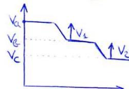
$$V_{ext} = V_1 + V_2 = IR_1 + IR_2 = I(R_1 + R_2)$$
